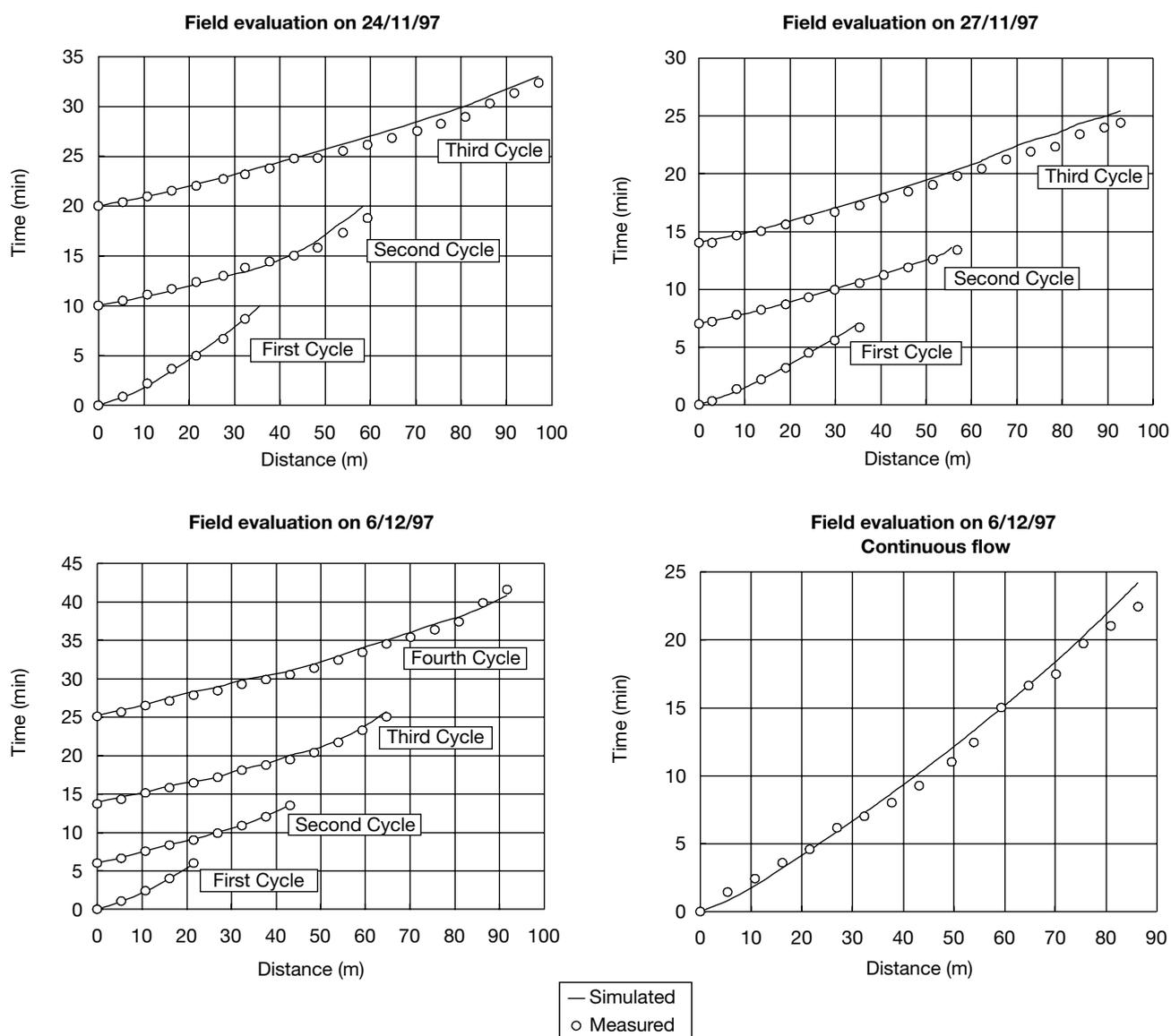
**Figure 3.** Comparison between measured advance curves and those obtained with the SIRMOD model.
