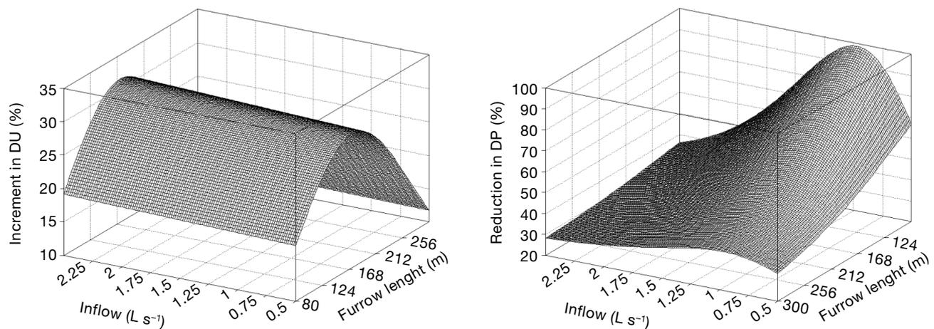
**Figure 8.** Increased distribution uniformity (left) and reduction in deep percolation losses (right) obtained when continuous flow irrigation is compared with surge irrigation.
