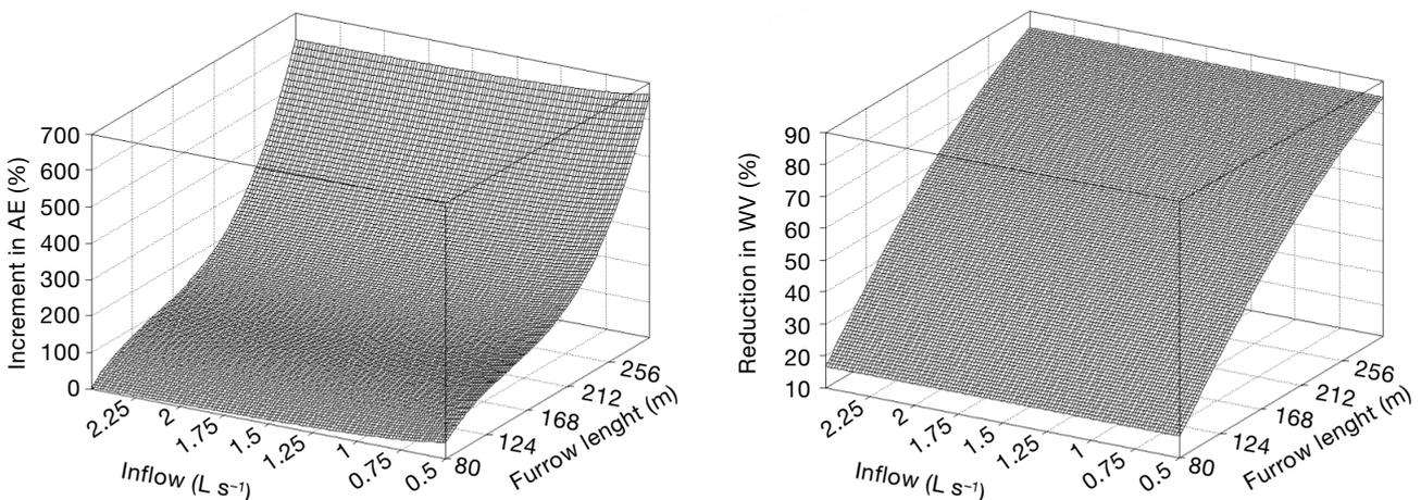
**Figure 7.** Increased application efficiency (left) and reduction in volume of water applied (right) obtained when comparing continuous flow irrigation with surge irrigation.
