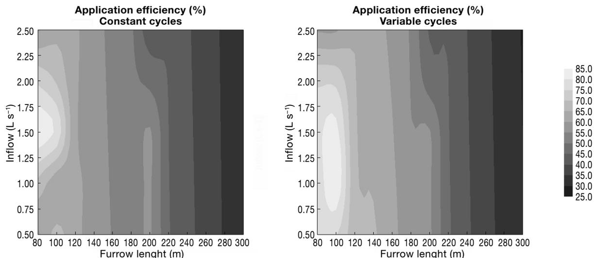
**Figure 5.** Contour lines of application efficiency obtained for constant cycle surge irrigation management strategies (left) and variable cycles (right).
