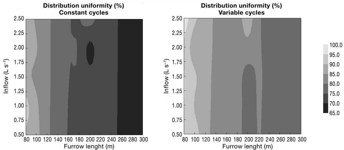
**Figure 6.** Contour lines of distribution uniformity obtained for constant cycle surge irrigation management strategies (left) and variable cycles (right).
