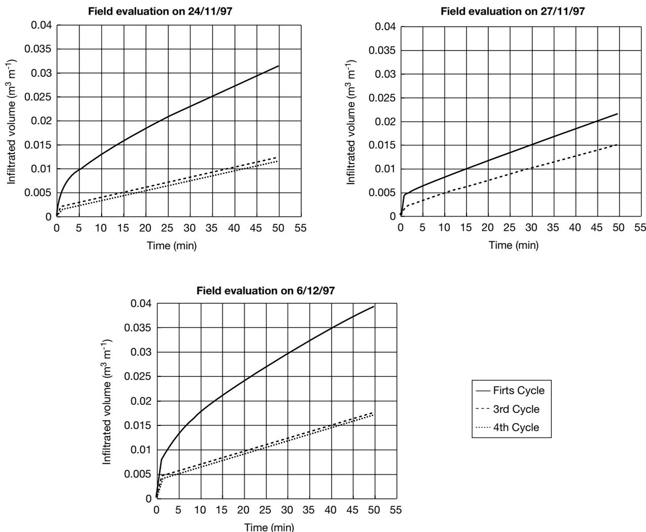
Figure 2. Volumes of infiltrated water for cycles 1, 3 and 4 obtained in surge irrigation evaluations.
